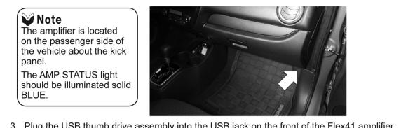
3. Plug the USB thumb drive assembly into the USB jack on the front of the Flex41 amplifier. The amplifier is located on the passenger side of the vehicle above the kick panel.
