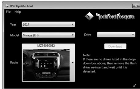
5. Insert a flash drive into the USB port of the computer and wait for the associated drive letter to be displayed in the "Drive" dropdown.
