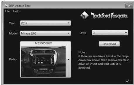
6. Press the "Download" button and then press "OK" to confirm that all files will be erased on the flash drive.
